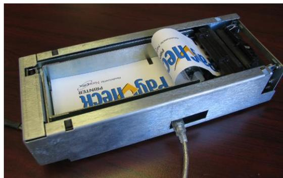
Figure 1 - Paycheck 3 printer with a USB cabled plugged in to the side USB port
