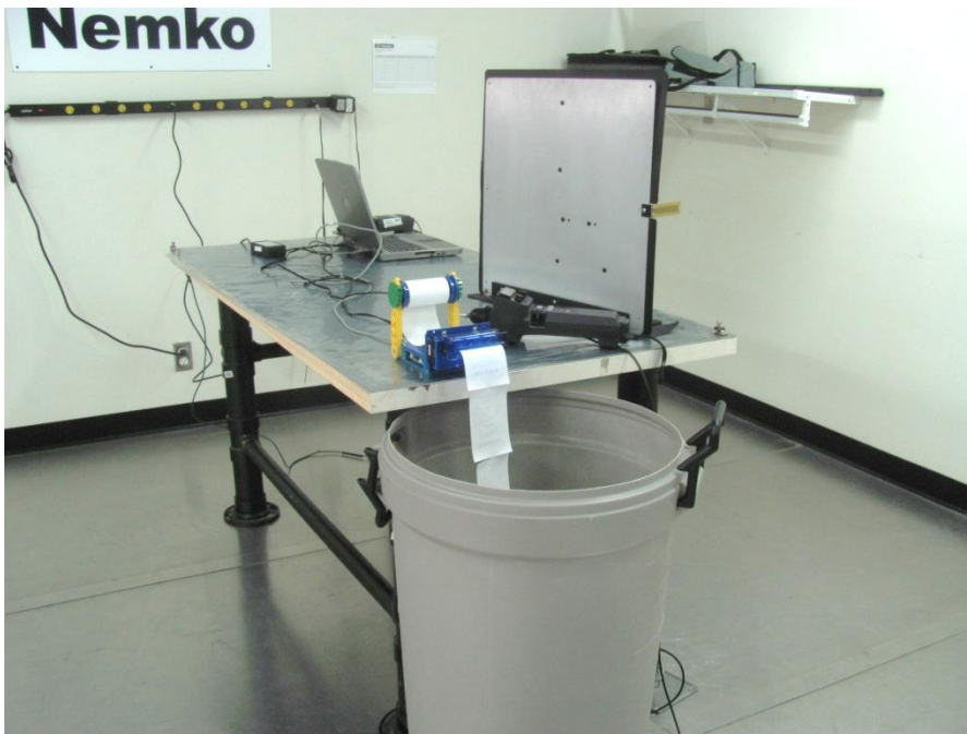
Photo 8.3-2: Electrostatic discharge setup
