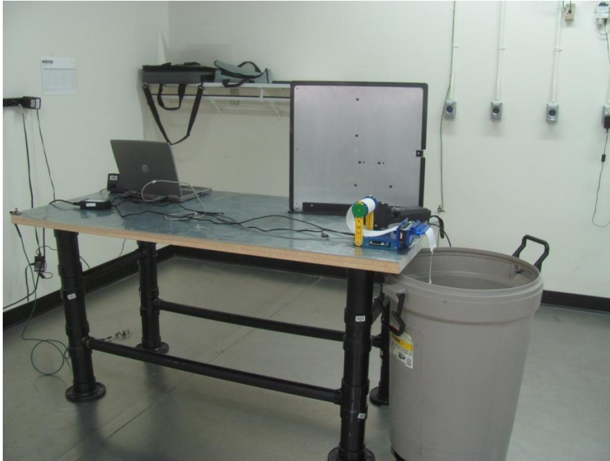
Photo 8.3-1: Electrostatic discharge setup
