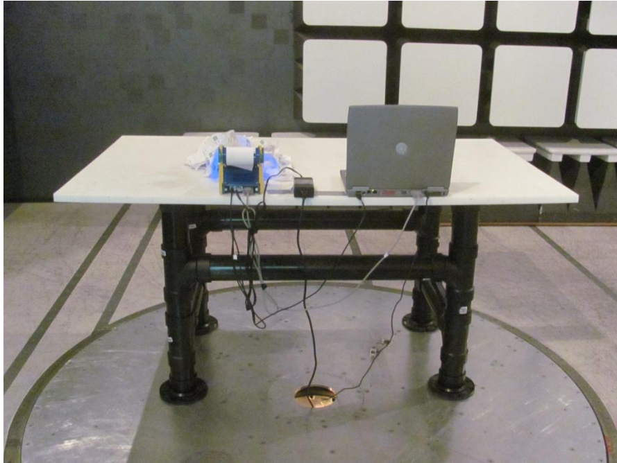
Photo 8.1-2: Radiated disturbance setup
