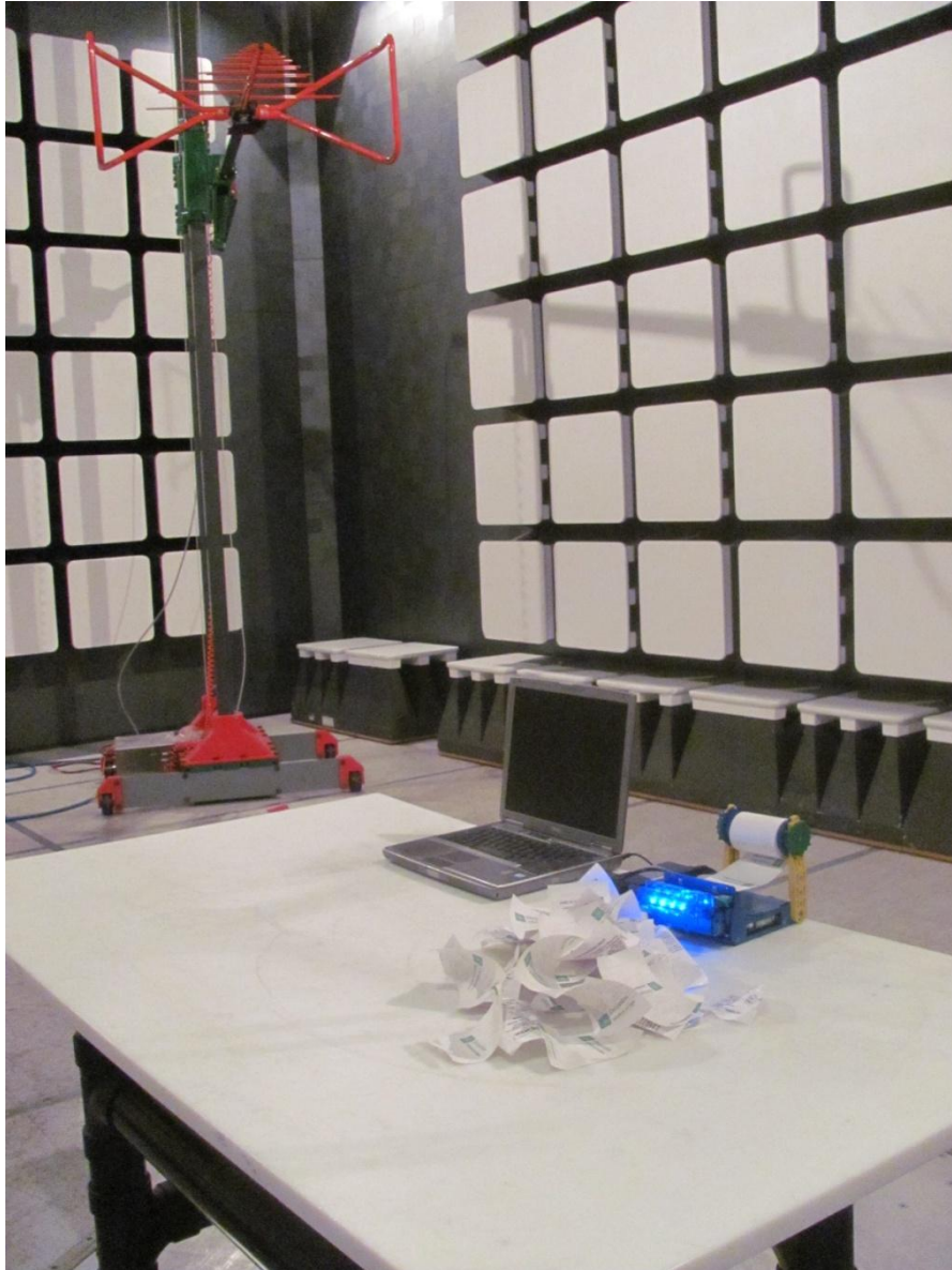
Photo 8.1-1: Radiated disturbance setup
